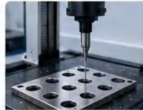
Dimension Inspection CMM full dimension inspection ensure precise tolerance
