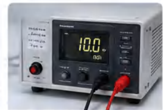
Electrical Insulation Test Dielectric strength and insulation resistance performance test
