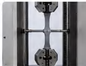
Tensile Strength Test Material tensile strength and elongation performance test
